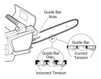
Figure 6 - Saw Chain Adjustment
